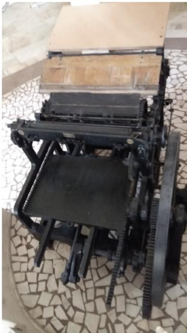
Printing press assembled from the pieces found in a scrap deposit in Germany
